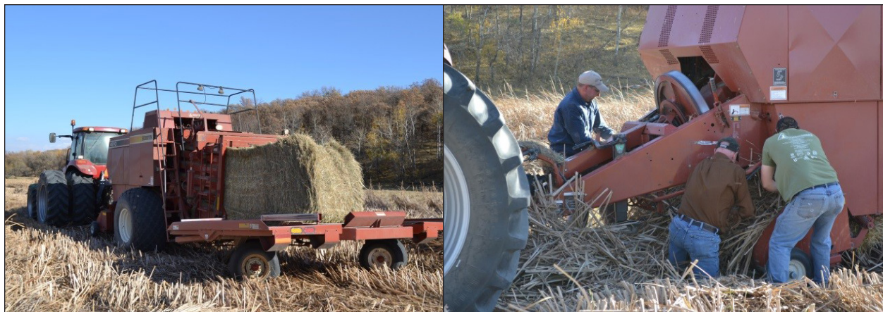
FIGURE 11. SQUARE BALER WITH SINGLE CATTAIL BALE STUCK IN BALER, AND PLUGGED THROAT OF BALER.
