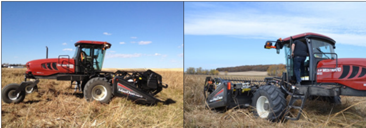
FIGURE 4. MACDON INDUSTRIES LTD WINDROWER USED FOR CUTTING STANDING CATTAILS AT ALL TEST SITES.
