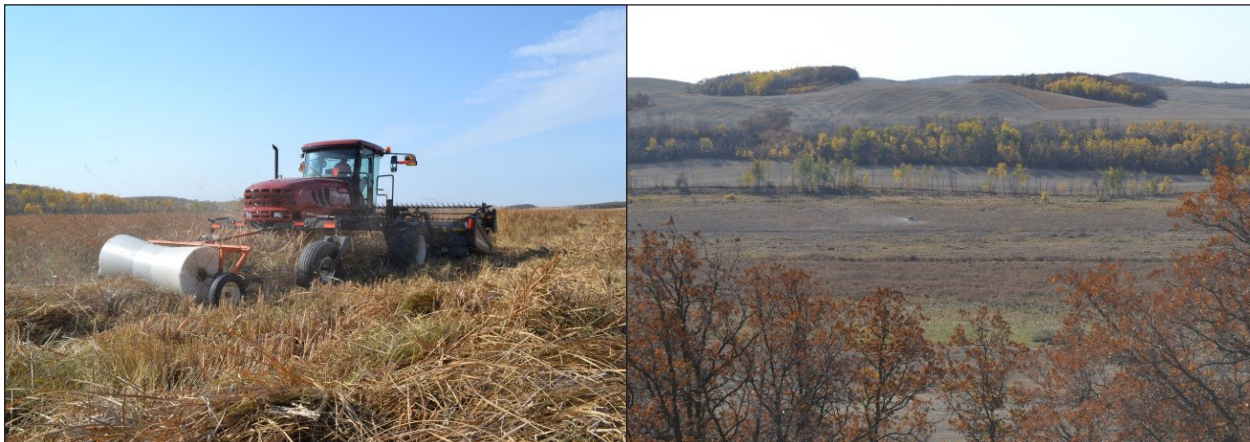
FIGURE 9. MACDON INDUSTRIES LTD WINDROWER CUTTING CATTAILS AT PELLY'S LAKE WETLAND. RIGHT IMAGE SHOWS WINDROWER IN PELLY'S LAKE WETLAND.
