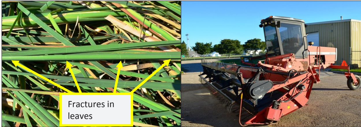
FIGURE 5. (LEFT) CRIMP MARKS LEFT BY CONDITIONER ROLLERS, AND (RIGHT) MASSEY FERGUSON MODEL 200 SWATHER
