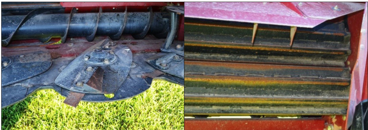
FIGURE 4. ROTARY CUTTING DISCS AND CONDITIONING ROLLERS ON THE MACDON R85 ROTARY DISC MOWER
