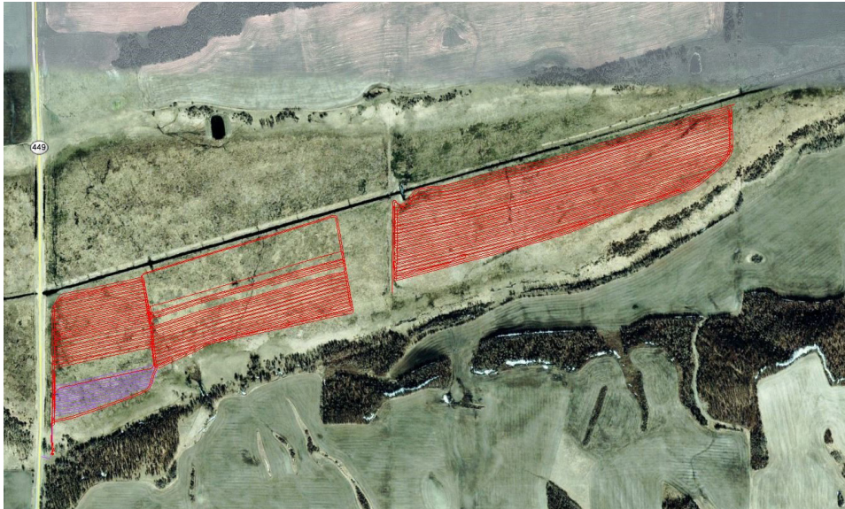
FIGURE 6. GPS TRACE OF THE MOWER WHILE CUTTING CATTAILS AT PELLY'S LAKE.
