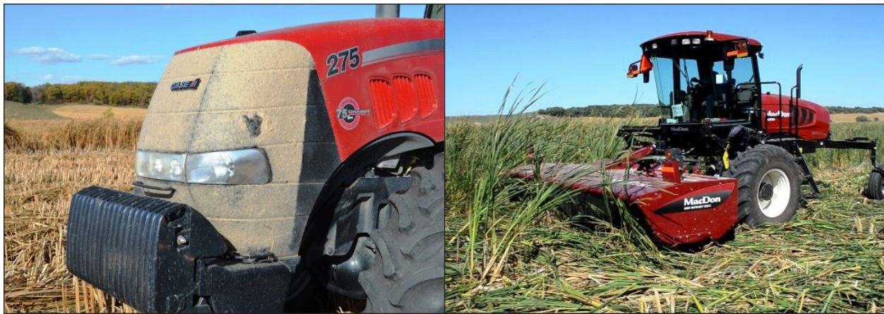
FIGURE 8. (LEFT) CATTAIL SEED FLUFF ON RADIATOR GRILL. (RIGHT) TRAMPLED AREA FROM LIVESTOCK.
