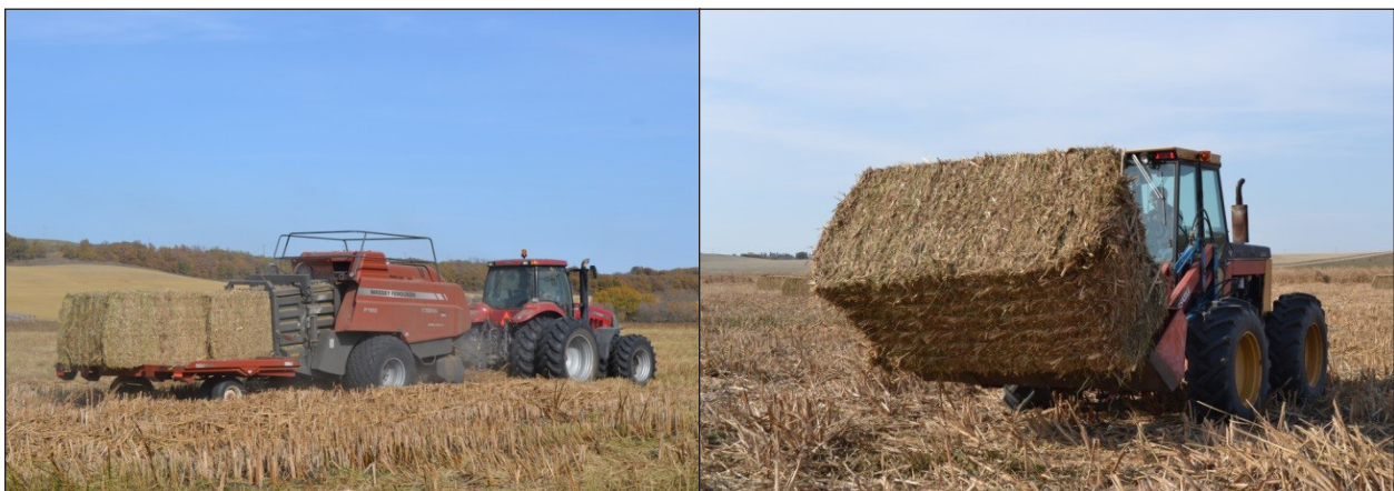
FIGURE 7. (LEFT) CASEIH MAGNUM 275 TRACTOR WITH MASSEY FERGUSON (HESSTON) 2190 SQUARE BALER. (RIGHT) LARGE SQUARE BALES PRODUCED FROM SWATHED CATTAIL (EACH WEIGHING APPROXIMATELY 1,500 LBS).
